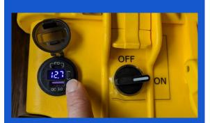
Turn on all units (2, 3 or 4) and check voltage on. Below 11.8V will require unit(s) to be charged\*
